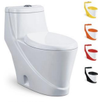
M-8036 Washdown One-piece Toilet Size: 690x380x700mm S-ramp: 250x200mm Roughing-in P-ramp: 180mm Roughing-in
