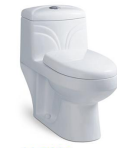
M-7035 Washdown One-piece Toilet Size: 700x380x700mm S-ramp: 250x200mm Roughing-in P-ramp: 180mm Roughing-in
