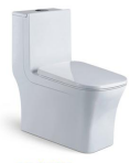
M-8124 Siphonic/Washdown One-piece Toilet Size: 670x370x700mm S-ramp: 250x200mm Roughing-in P-ramp: 180mm Roughing-in
