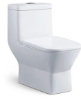
M-8104 Siphonic/Washdown One-piece Toilet Size: 650x370x700mm S-ramp: 250x200mm Roughing-in P-ramp: 180mm Roughing-in
