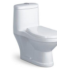
M-0035 Children Washdown One-piece Toilet Size: 470x380x700mm S-ramp: 100mm Roughing-in P-ramp: 120mm Roughing-in
