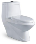
M-8126 Washdown One-piece Toilet Size: 760x410x750mm S-ramp: 250x200mm Roughing-in P-ramp: 180mm Roughing-in
